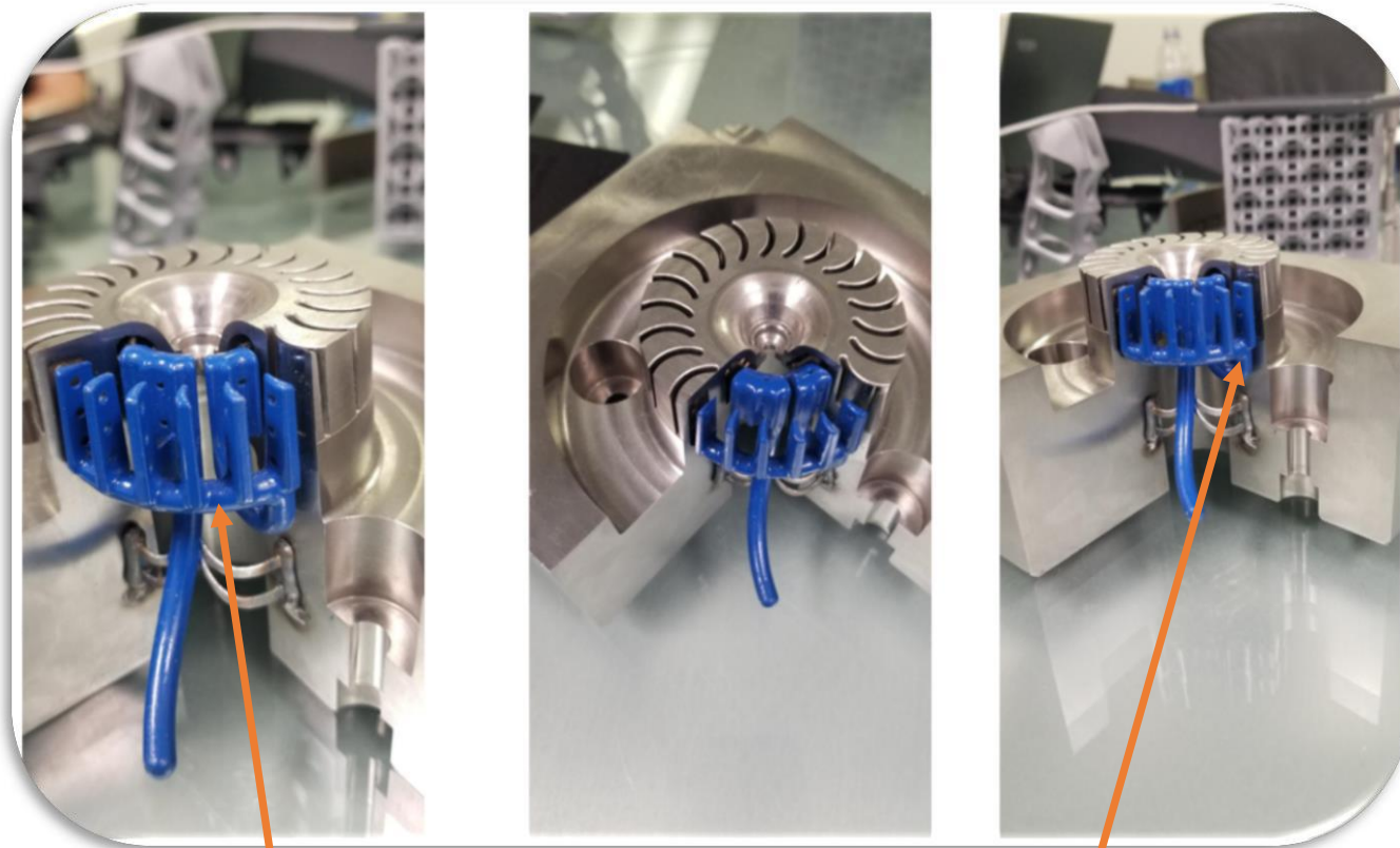
Blue Represents Conformal Cooling Channels Not Possible with Conventional Machining
